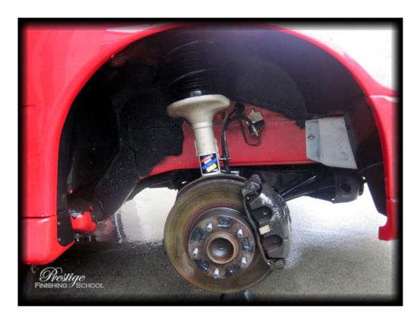
Although an underseal has been applied to the bulk of the wheel arches, a small plastic liner is still fitted – this is dressed with Meguiars All Season Dressing, leaving a very smart finish.
